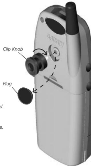
1. Remove the plug from the back of the NavTalk unit.
