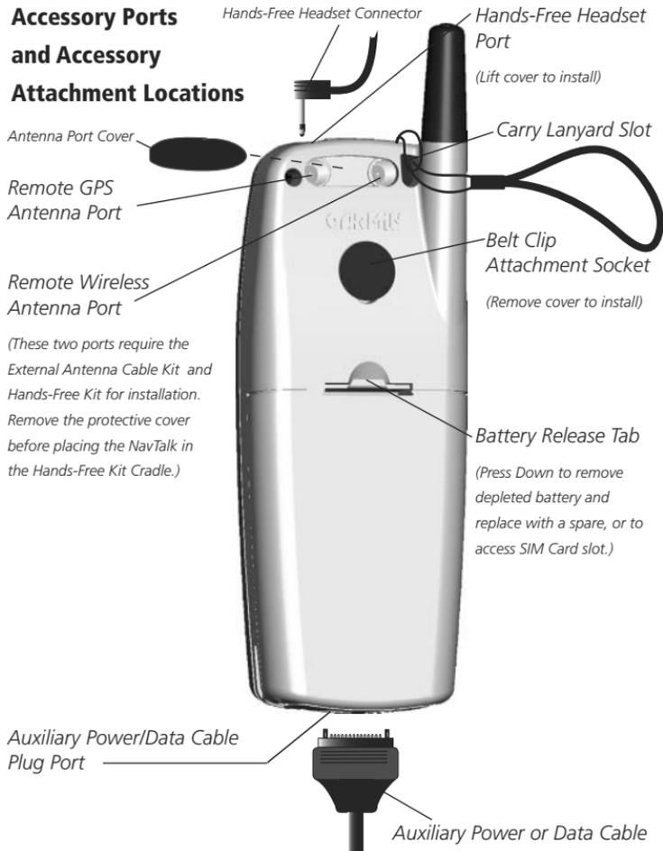
*(These two ports require the External Antenna Cable Kit and Hands-Free Kit for installation. Remove the protective cover before placing the NavTalk in the Hands-Free Kit Cradle.)*
